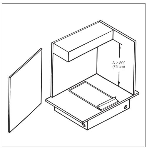
To reduce the risk of fire or burns caused by reaching over heated surface units, locating cabinet storage space above these units should be avoided.
